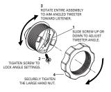
**Note:** Check screw clearance before installing. Use glue if clearance is an issue.
